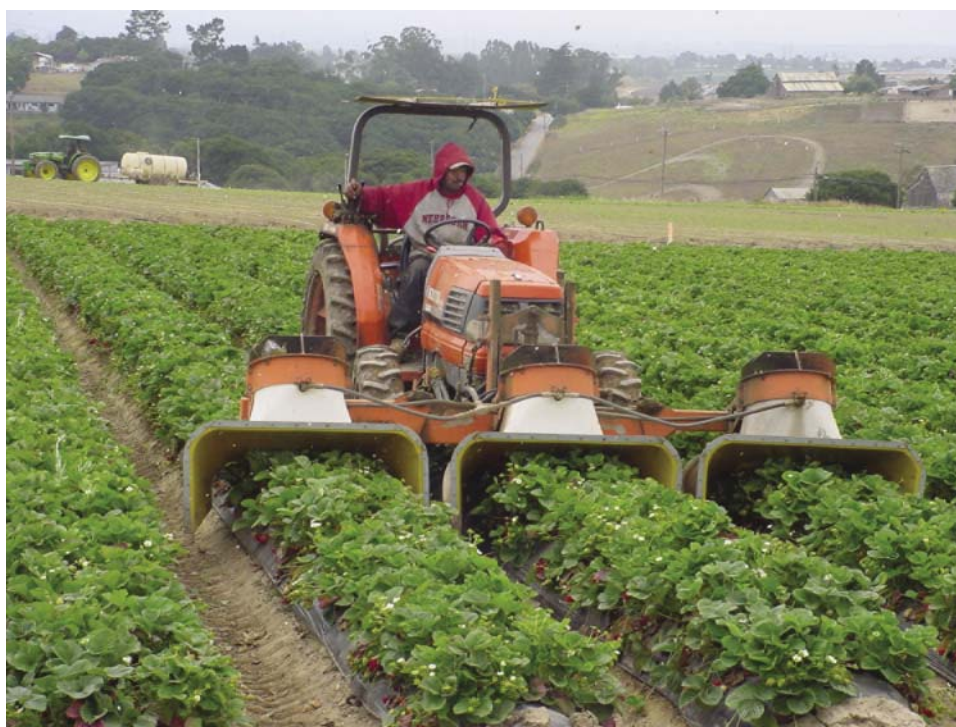
A Bug-Vac moves through a strawberry field. Aphids and other small, winged insects can move into organic fields and quickly reach damaging levels. Machines have been developed that use suction to capture and remove these insects.
